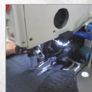
Reflective tape is uncovered - the lapel buttonhole is sewn
