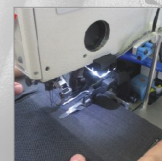
Reflective tape is covered - the front buttonholes are sewn
