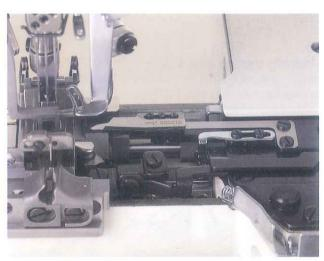
Thread Trimmer This device eliminates the use of scissors allowing you to concentrate on sewing operation. The result is a boosted efficiency.
