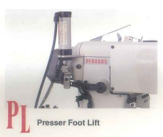
The presser foot can be lifted pneumatically with heel treadle. Ease of operatoin decreases operators fatigue.
