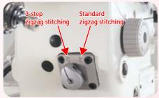
Standard/3-step zigzag stitching pattern changeover lever
