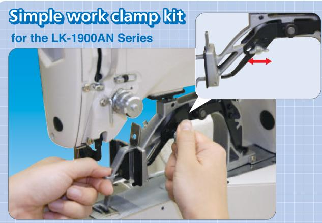
·Conventionally, the front plate has to be removed to change the work clamp. With the new work clamp kit, the work clamp can be changed without removing the plate.
