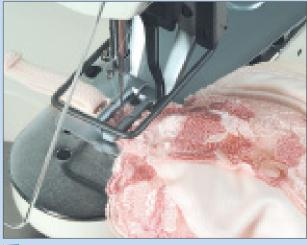
**F type** (Attaching the shoulder straps to brassier) \* Presser foot for vertical bartacking is supplied with the unit as an accessory.
