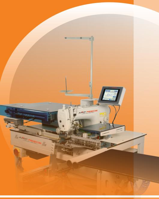
Even inexperienced operators can create high quality and accurate dart seams and pleats by adjusting the desired length, depth and angle from the user friendly touch screen display. Different specifications of darts and pleats can easily be programmed on the 10 preset memories. The operator can cycle between 4 different dart and pleat sewing programs without having to change any gauge parts which makes the unit very flexible and productive.
